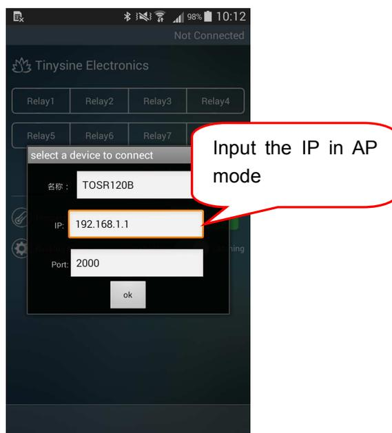
192.168.1.1 is the default IP address in AP mode, not the IP you configured based on your wireless network. After your phone joins the network and verifies the password, you can control TOSR120B as usual!
