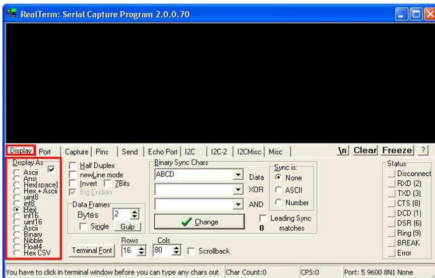
(3) Input the commands you want to send in option “ **Send** ”, but Realterm can only send data as **Dec** or **Hex**, here we choose Dec for demo. No matter which way you choose, the first thing before you can control TOSR120B is to verify the password!
