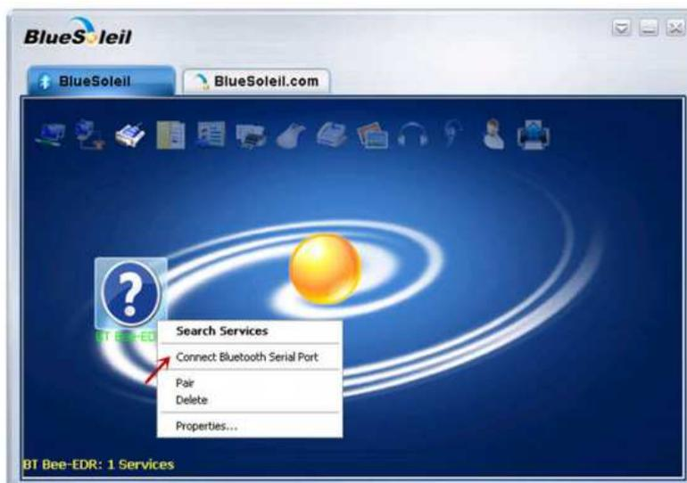
(6) Once your computer has connected with Bluetooth Bee V2, the “ **STATE** ” led stops blinking. Meanwhile, the device turns green and BlueSoleil shows “ **Connected** ”.
