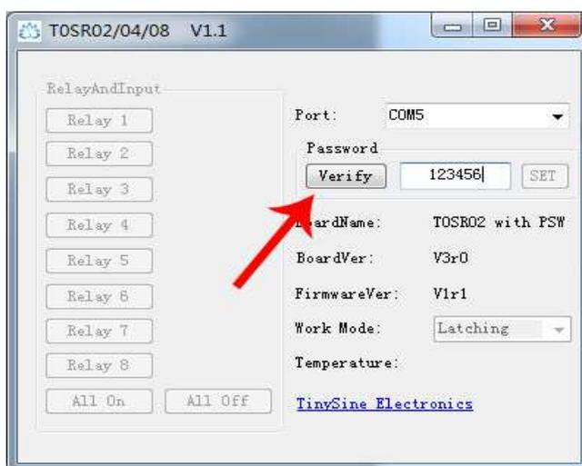
(3) After inputting the correct password, all the buttons become enabled, then you can control the board now!
